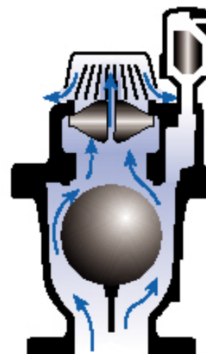
Air outflow through reduced orifice
